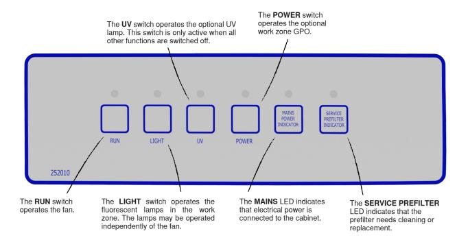
PCR Series cabinets are fitted with a low-voltage, touch-control panel to operate standard cabinet functions a general purpose power outlet (GPO) and ultraviolet (UV) lamp.
